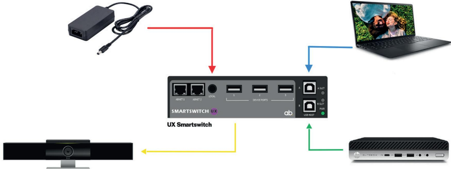
If used in Standalone mode (without a TX2 / DX2) you will require the optional power supply (part no. 900-00585) to power the UX.
