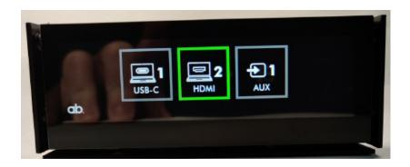
Provides a set of 3 buttons for the selection of the USB-C and HDMI inputs in the VXT and the Aux 1 HDMI input on the VXR.
